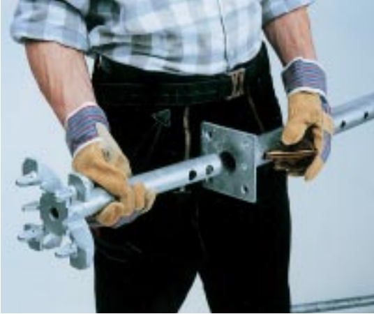
Above: The connection of TOPEC bearing and prop: Slip on the bearing, press in the spring bolt—that's all there is to it.
